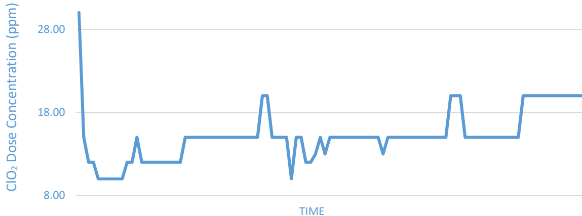
Figure 1. A Typical Job Log: ClO 2 Dose Delivered as a Function of Time
